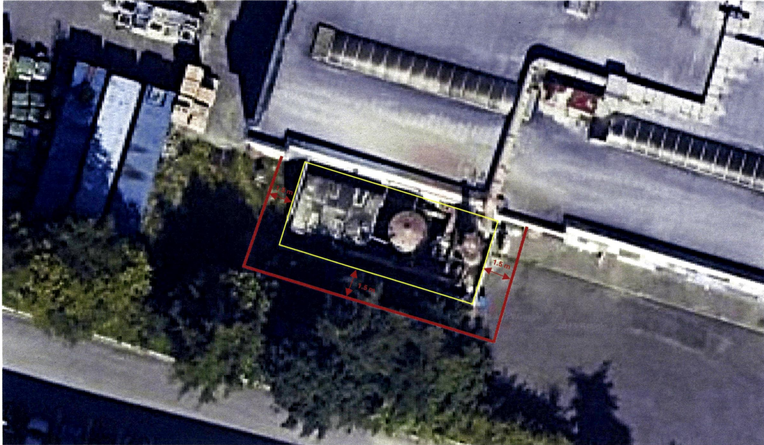
Figure 2: Proposed abatement system soundproof housing extension. Yellow line outlines current bund wall. Red line outlines proposed housing unit extension perimeter.
